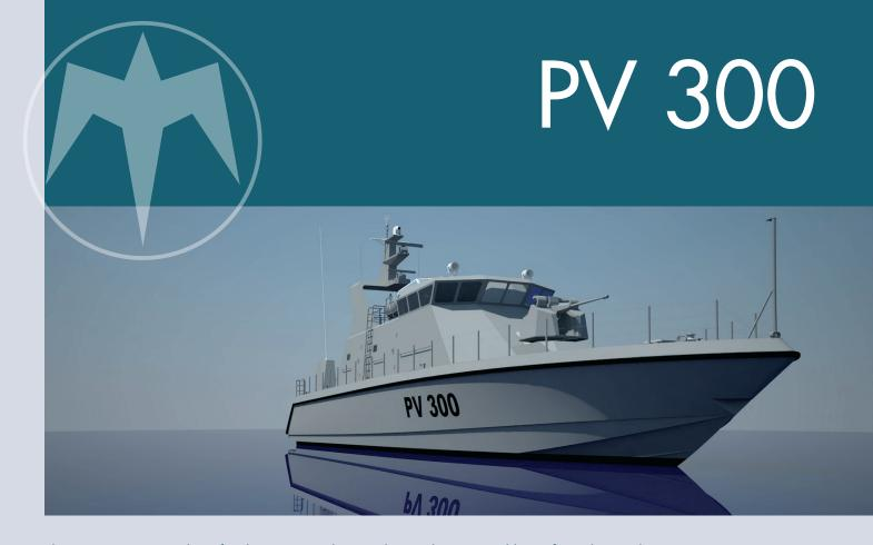
The PV300 is a 33 m long fast boat in GRP that can be used as a patrol boat, for police and rescue operations. It is highly customisable in terms of propulsion and interior layout and features.
